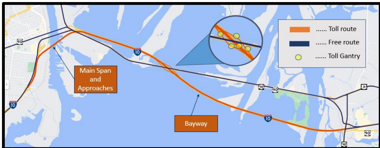
Figure 3: Proposed Toll Gantry Locations at Mid-Bay Interchange
