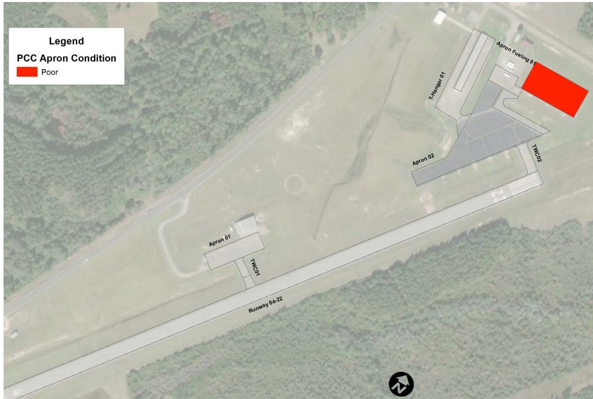
Figure 3.4: PCC Apron Condition Rating.
