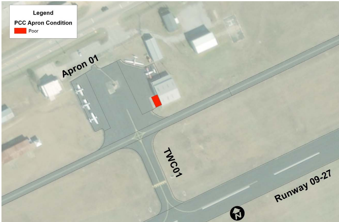
Figure 3.4: PCC Apron Condition Rating.
