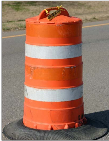
X Sheeting Too Narrow (6" Minimum Required)
