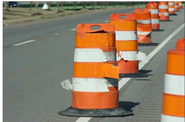
X Sheeting in Poor Condition
