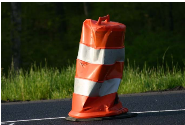
X Damage to Drum Shape
