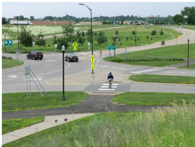
Example of a multi-lane roundabout.
