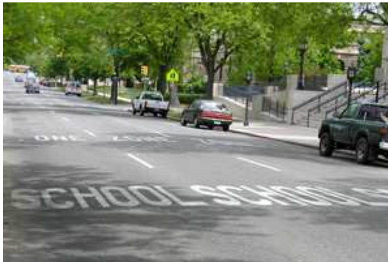
Figure 29. School Zone Pavement Markings
