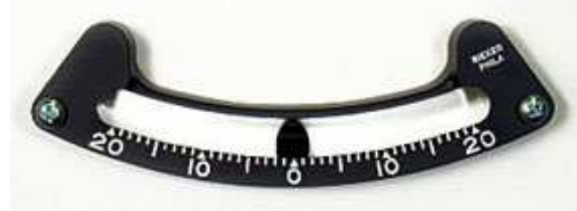
Example of a Ball Bank Indicator
