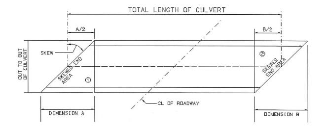
Calculate the reinforcing steel quantity for the total length of the culvert using the quantities shown on the standard drawing and add the following amounts for the skewed end areas:
