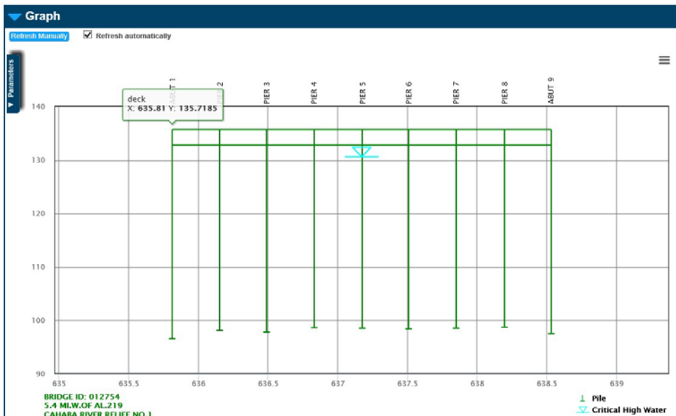
Figure 104 – Graph with structure detail plotted
