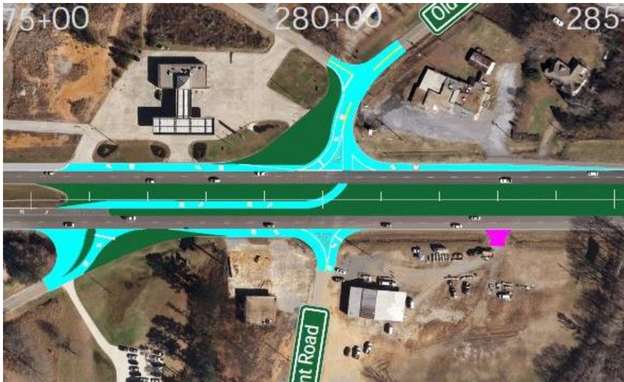
Figure E-21: Proposed Improvements at Main Intersection
