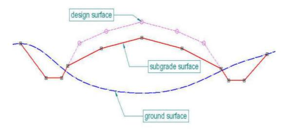
From the Design Surface palette, choose Merge Surfaces and set Original Surface: design, Design Surface: subgrade, Target Surface: default. Uncheck all boxes and choose Apply.
