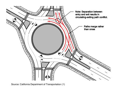
Exhibit 6-34 illustrates a possible low-cost fix that involves modifications to the lane arrangements using a combination of striping and physical modifications. This may be acceptable if the traffic volumes are compatible. A better solution is illustrated in Exhibit 6-35, which involves realignment of the approach legs to have the paths of entering vehicles cross the paths of the circulating traffic (rather than merging) to eliminate the conflict.
