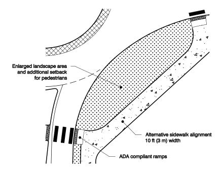
The recommended sidewalk width at roundabouts is 6 ft (1.8 m), and the minimum width is 5 ft (1.5 m). In areas with heavy pedestrian volumes, sidewalks should be as wide as necessary to accommodate the anticipated pedestrian volume. At any roundabout where ramps provide sidewalk access to bicyclists, the sidewalk should be a minimum of 10 ft (3 m) wide to accommodate shared use by pedestrians and bicyclists. An example of sidewalk setback is given in Exhibit 6-65.
