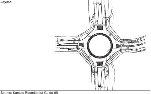
Exhibit 8-6 Example of Illumination Using Cobra-Style Luminaires
