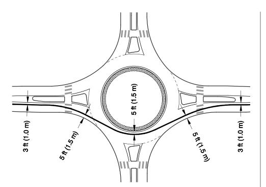
**Exhibit 6-48**Fastest Vehicle Path through Single-Lane Roundabout
