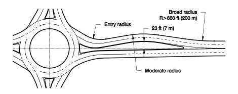
Right-turn bypass lanes can be used in locations with minimal pedestrian and bicycle activity to improve capacity when heavy right-turning traffic exists.
