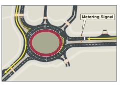
Metering signal briefly stops traffic from the east, which allows traffic from the north to enter the roundabout.
