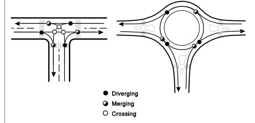
A four-leg single-lane roundabout has 75% fewer vehicle conflict points and no crossing conflict points compared to a conventional intersection. Exhibit 5-2 presents similar diagrams for a conventional four-leg (X or cross) intersection and a four-leg roundabout. As the figure shows, the number of vehicle-vehicle conflict points for roundabouts decreases from thirty-two to eight with four-leg intersections.
