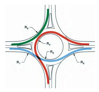
Recommended maximum theoretical entry design speeds for roundabouts at various intersection site categories are provided in Exhibit 6-47.
