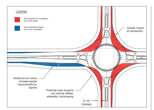
**Exhibit 3-17**Area Comparison: Single-Lane Roundabout versus Comparable Signalized Intersection
