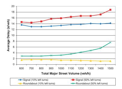
**Exhibit 3-19**Average Control Delay per Vehicle at the MUTCD Peak-Hour Signal Warrant Thresholds
