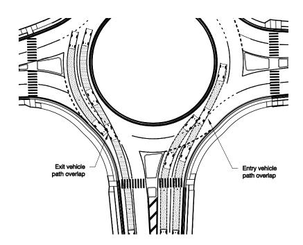
upon the exit from the roundabout where the exit radii are too small or the overall exit geometry does not adequately align the vehicle paths into the appropriate lane. Additional information on entry and exit design at multilane roundabouts is provided in Section 6.5.
