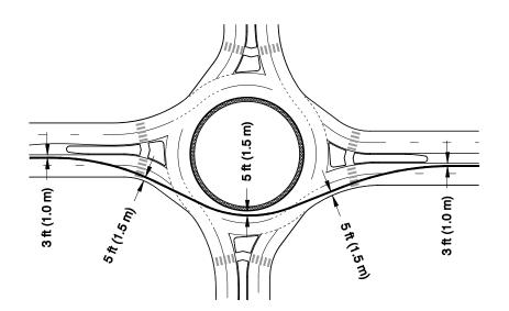
**Exhibit 6-49**Fastest Vehicle Path through Multilane Roundabout
