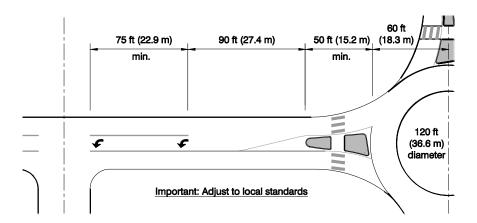
Sight distance needs. A driver at the access point should have proper intersection sight distance and should be visible when approaching or departing the roundabout, as applicable.
