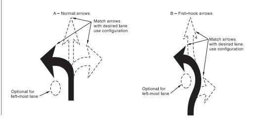
quickly lose their readability when a portion of the marking is worn away by the tires of passing vehicles.
