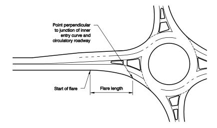
designs. Entry widths should therefore be minimized and flare lengths maximized to achieve the desired capacity with minimal effect on crashes.
