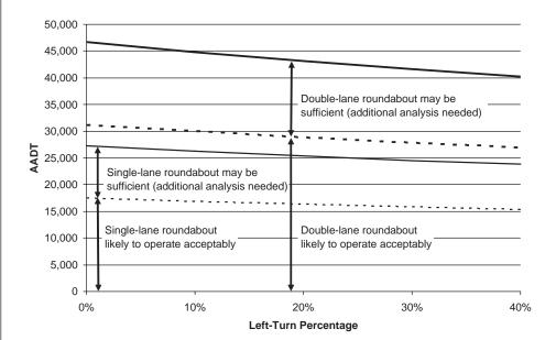
If the volumes fall within the ranges identified in Exhibit 3-12 where "additional analysis is needed," a single-lane or two-lane roundabout may still function quite well, but a closer look at the actual turning-movement volumes during the design hour is required. The procedure for such analysis is presented in Chapter 4.
