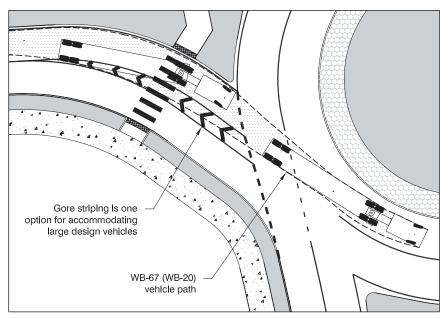
**Exhibit 6-37**WB-67 (WB-20) Truck Path with Gore Striping at Entry
