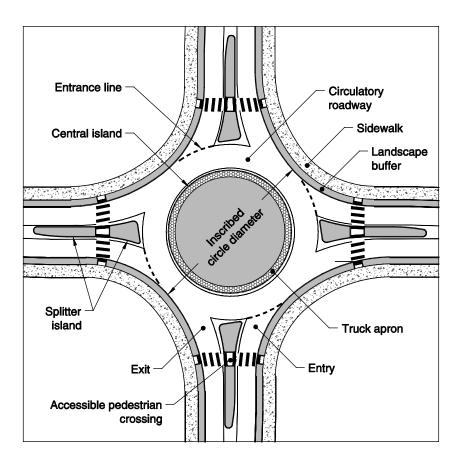
**Exhibit 6-2**Basic Geometric Elements of a Roundabout
