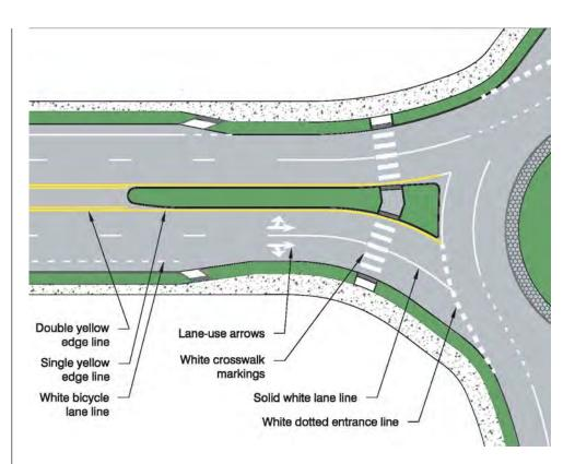
double yellow lines. For small splitter islands [area less than 75 ft² (7 m²)], the island may consist of pavement markings only, in the form of two sets of double yellow lines or marking the entire splitter island yellow. However, raised splitter islands should be used where possible.
