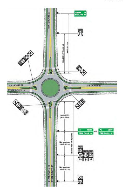
**Exhibit 7-25**Example Sign Layout for Guide Signs at Roundabouts
