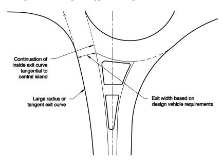
At single-lane roundabouts in urban environments, exits should be designed to enforce slow exit path speeds to maximize safety for pedestrians crossing the exiting traffic stream. Pedestrian activity should be considered at all exits except where separate pedestrian facilities (grade separated paths, etc.) or other restrictions eliminate the likelihood of pedestrian activity in the foreseeable future.
