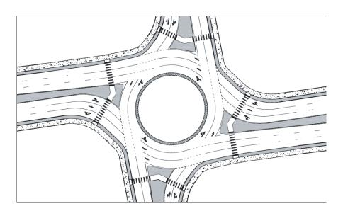
As discussed previously for single-lane roundabouts, a useful surrogate for capturing the effects of entry speed, path alignment, and visibility to the left is entry angle (phi). Typical entry angles are between 20° and 40°. Additional detail on entry angle can be found in the Wisconsin Department of Transportation *Roundabout Guide* (7) and design guidance from the United Kingdom (9, 10).
