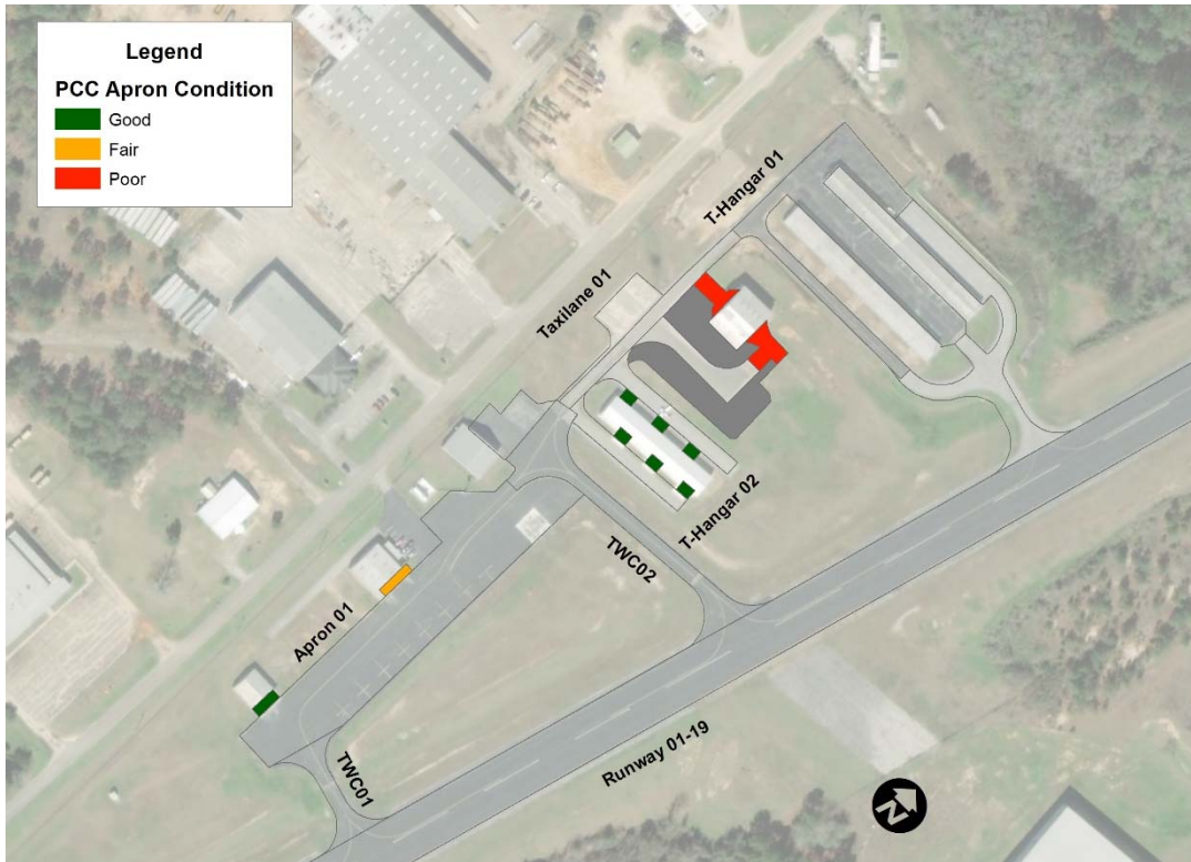
Figure 3.4: PCC Apron Condition Rating.
