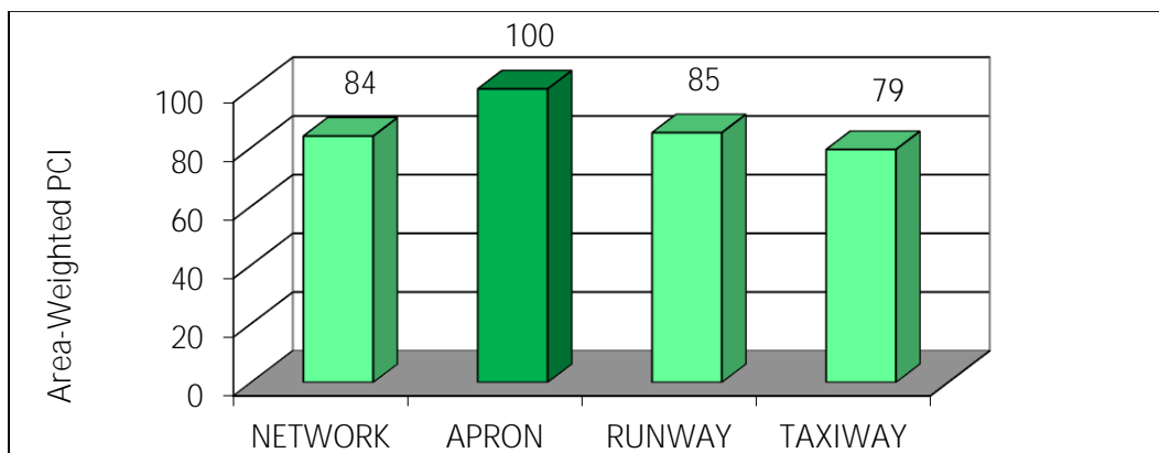
Figure 3.2: Pavement Condition by Branch Use.
