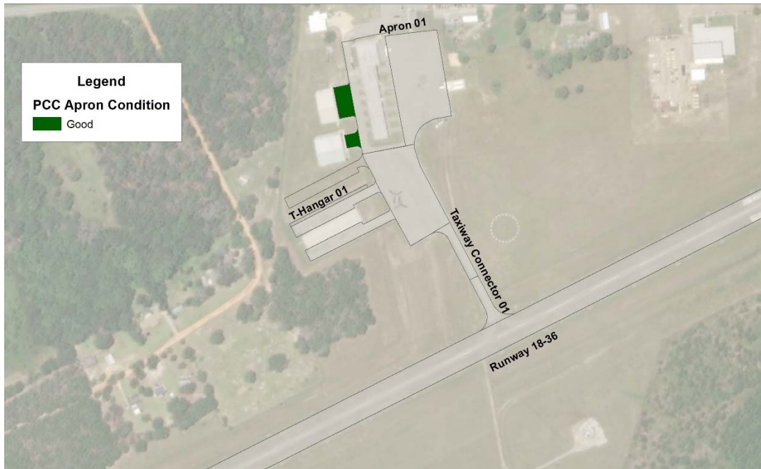
Figure 3.4: PCC Apron Condition Rating.
