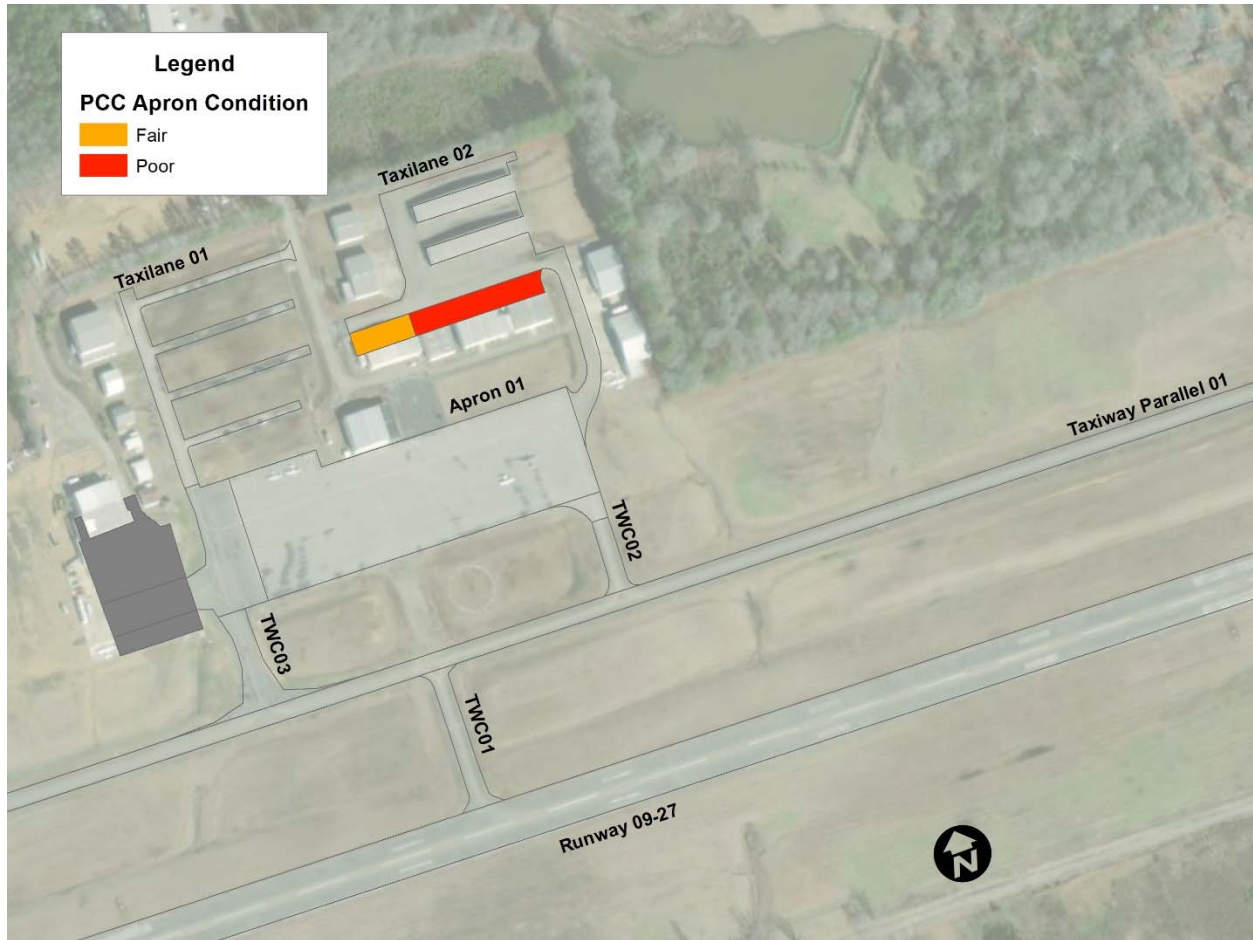
Figure 3.4: PCC Apron Condition Rating.
