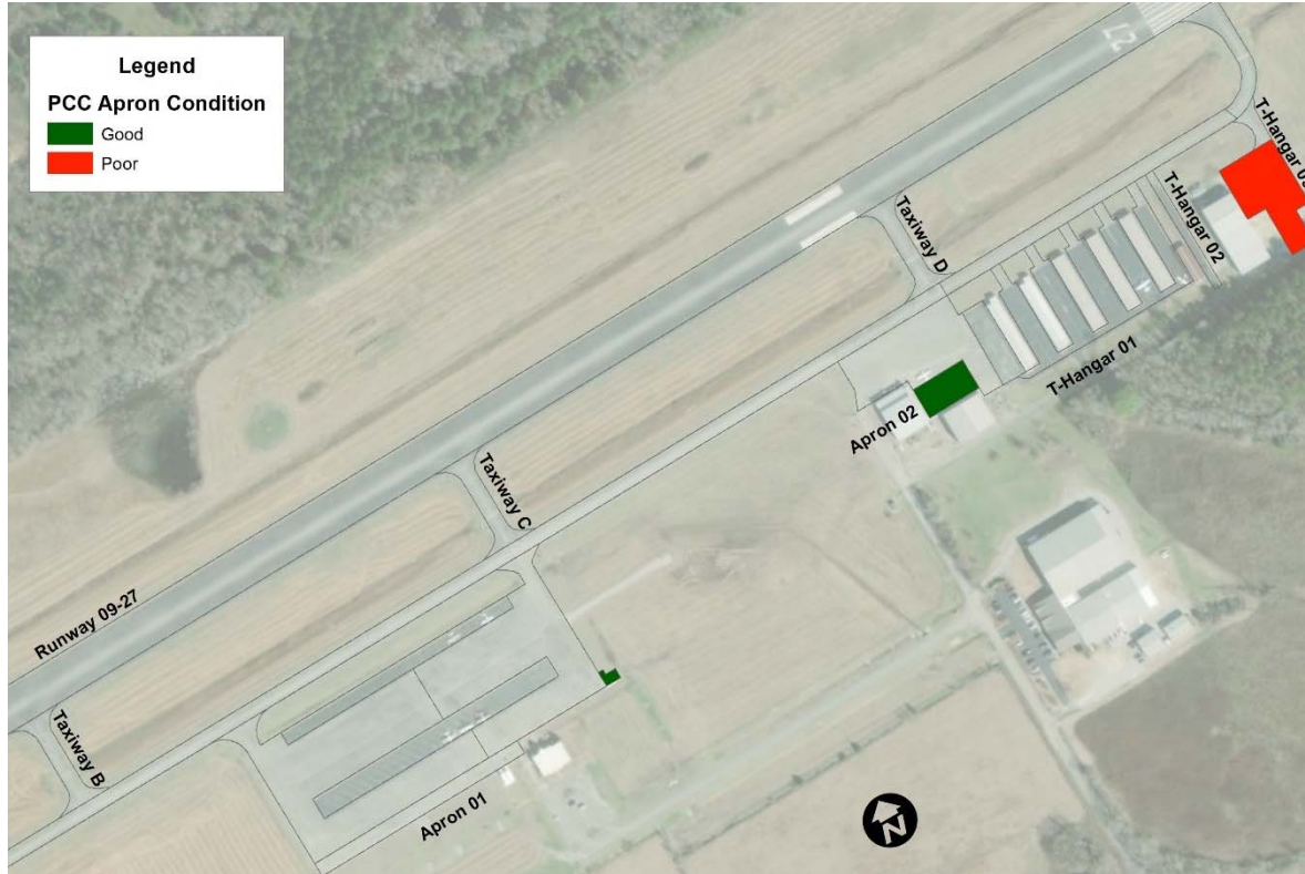
Figure 3.4: PCC Apron Condition Rating.
