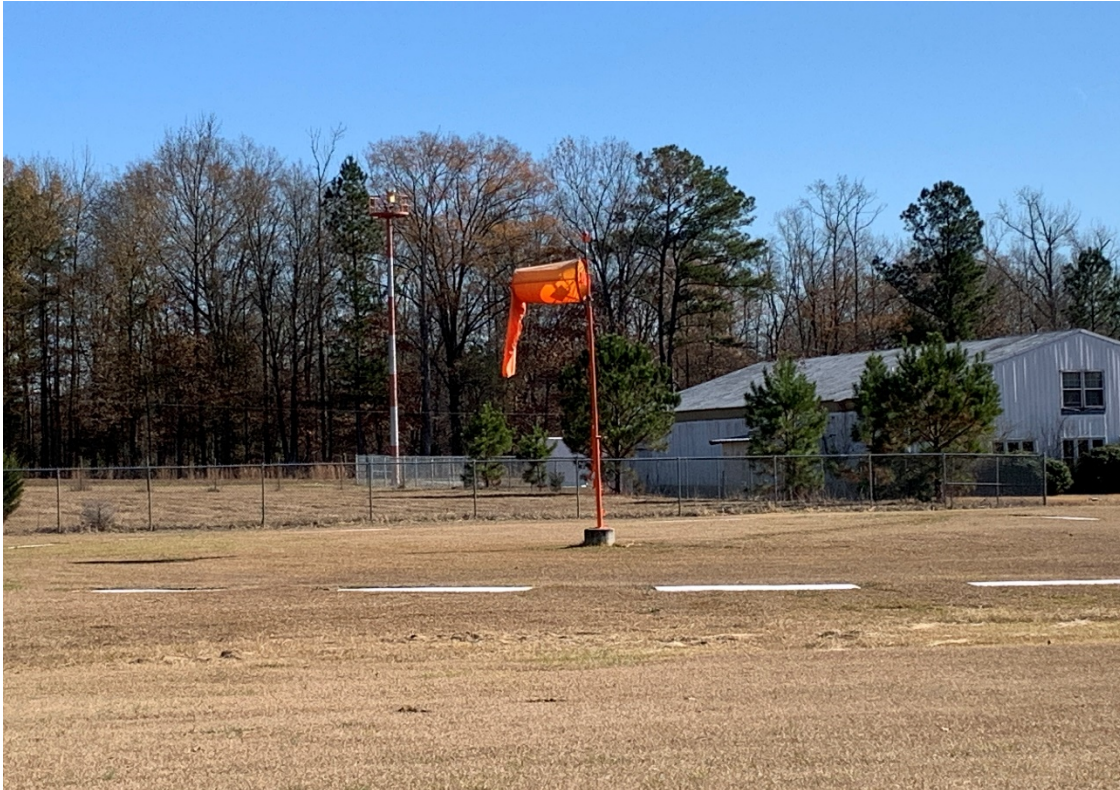
Photo #5 – Wind Direction Indicator
