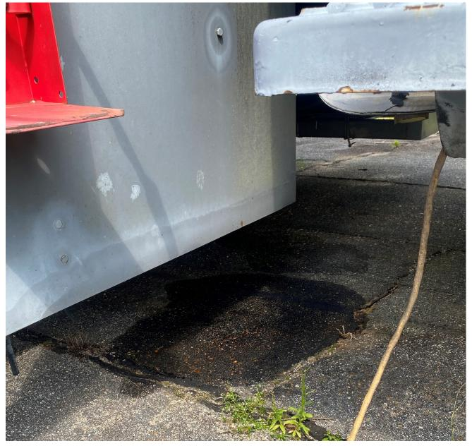
One of the fuel trucks is leaking fuel onto the ground contaminating the soil underneath. Also, the State of Alabama Department of Agriculture may have additional requirements for fueling systems that were not considered during this inspection.
