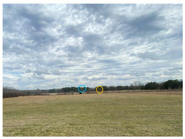
No obstructions were located in the ALDOT Approach/ Departure Path of Runway 27. The tree circled in blue penetrates the FAA Part 77 Approach Path. The tree circled in orange creates a 20:1 slope and is expected to penetrate the ALDOT Approach/Departure Path soon. Please see Appendix 3 for more information.
