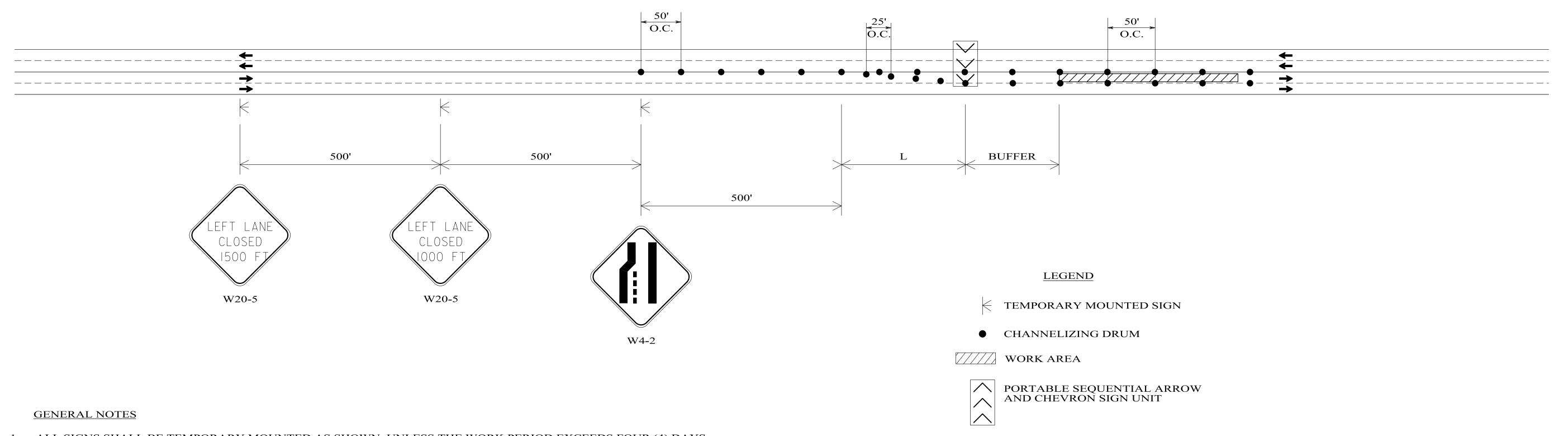
1. ALL SIGNS SHALL BE TEMPORARY MOUNTED AS SHOWN, UNLESS THE WORK PERIOD EXCEEDS FOUR (4) DAYS. IN SUCH CASES, THE SIGNS SHALL BE POST MOUNTED.
