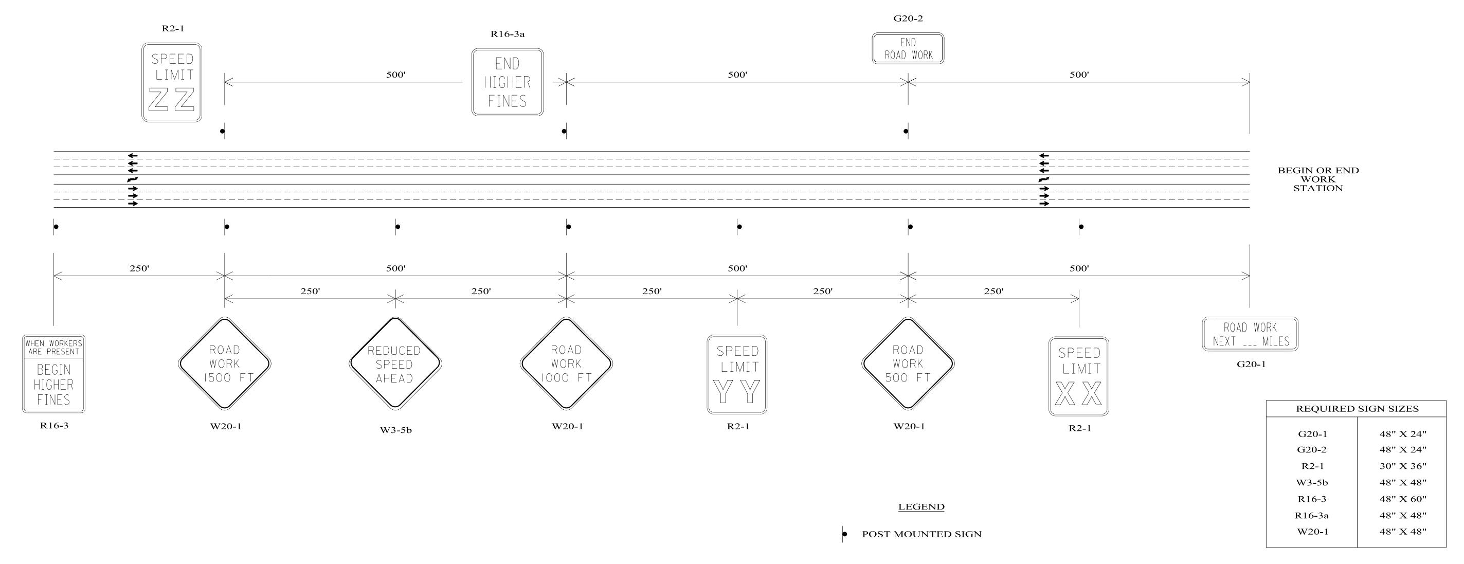
THE SIGN SIZES SHOWN ON THIS SHEET SHALL SUPERCEDE THOSE SHOWN ON THE STANDARD HIGHWAY SIGNS DRAWINGS UNLESS OTHERWISE APPROVED BY THE ENGINEER.
